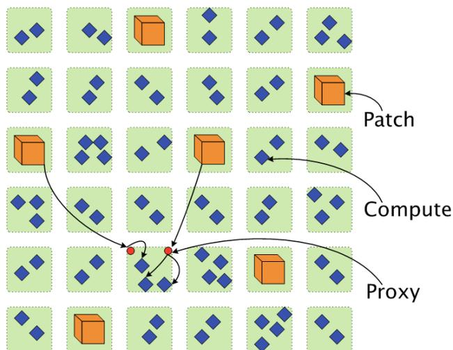
**Figure 2: Placement of patches, computes and proxies on a 2D mesh of processors**
