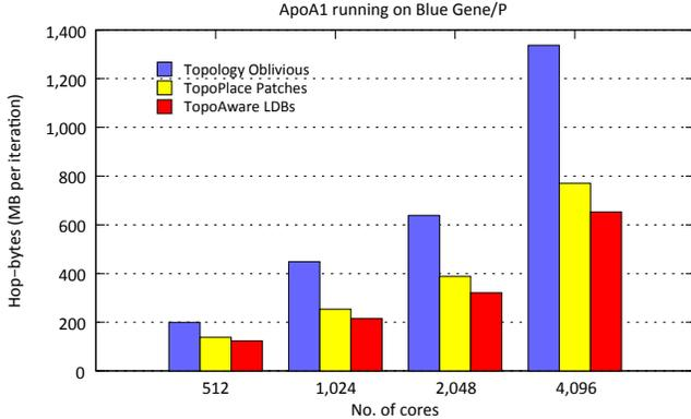
Figure 5: Hop-bytes for different schemes on IBM Blue Gene/P
