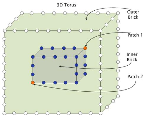
**Figure 4: Topological placement of a compute on a 3D torus/mesh of processors**
