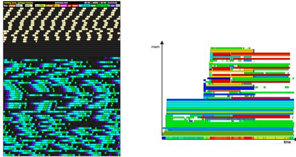
Figure 3: Left: Memory visualization by [GT89]. Memory address space depicted as a 1-dimensional array wrapping down several rows. Blocks indicate allocations along address space, color legend indicates variable data types. Printed with author’s permission. Right: Memory visualization by [MT07]. Allocations depicted as 2D blocks with address space on the vertical axis and time on the horizontal axis. Image courtesy of A. Telea.
