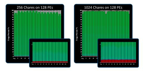
Application code in green, runtime overhead in red, idle time in white (Insets are enlargements of y-axes)
