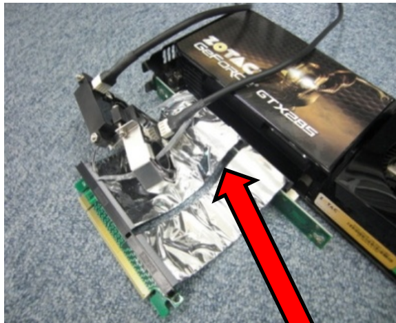
Attaches current sensors to two power lines in PCIe
