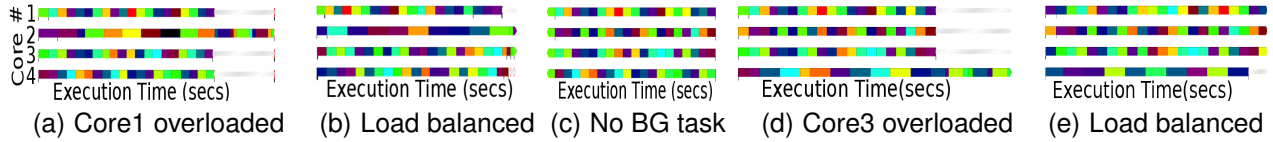
Figure 3: Cores timeline showing effect of load balancing for a 4 core run with background load on Core1 and then Core3
