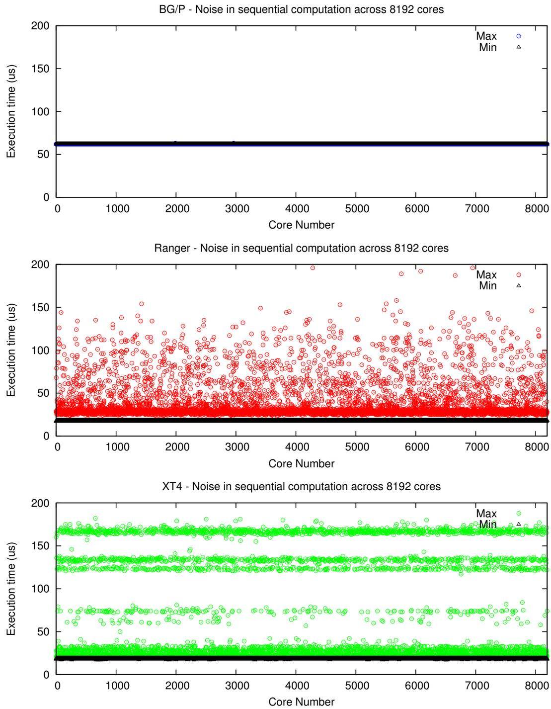
Figure 4: Plot showing system noise plotted against all ranks in a 8192-core run
