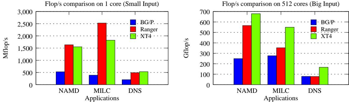
Figure 14: Flop/s comparisons of the three applications on BG/P, Ranger and XT4
