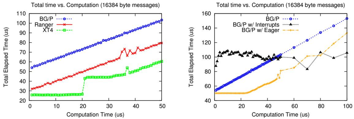
Figure 8: Results of the Communication-Computation Overlap benchmark for 16 KB messages (left) and various optimization possibilities on BG/P (right)
