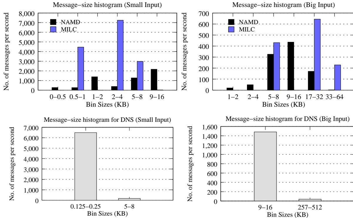
Figure 13: Message size histogram for the three applications on XT4 using 512 cores (average values per core)
