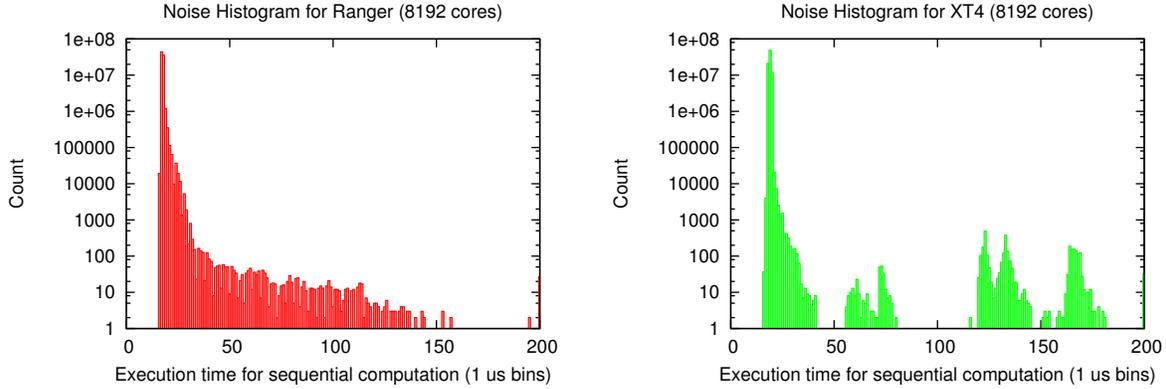
Figure 5: Histograms for the execution time of the sequential computation on Ranger and XT4
