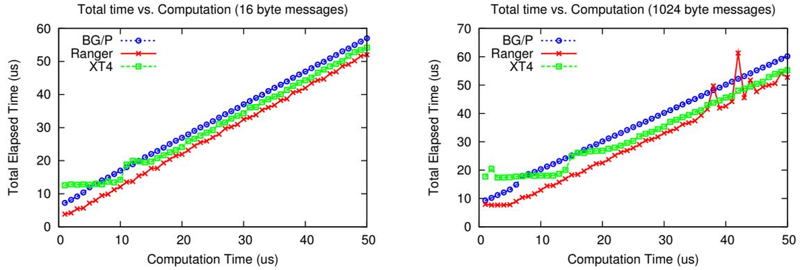
Figure 7: Results of the Communication-Computation Overlap benchmark for 16 and 1024 byte messages
