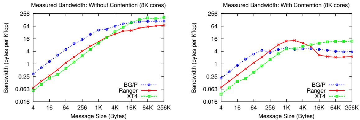
Figure 3: Bandwidth per flop/s comparisons using WOCON and WICON Benchmarks
