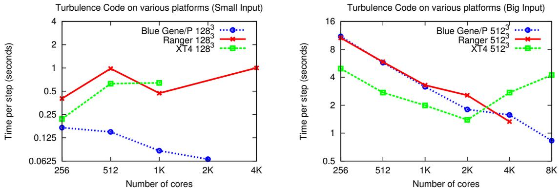
Figure 11: Performance (strong scaling) of DNS (Turbulence code) on the three machines
