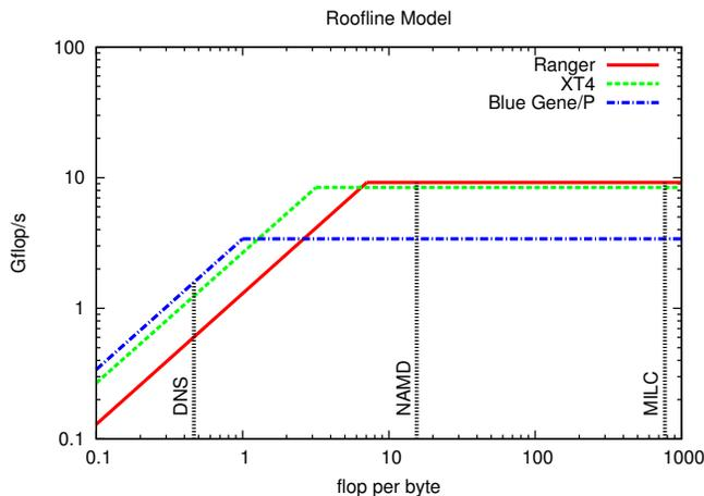
Figure 1: Roofline model
