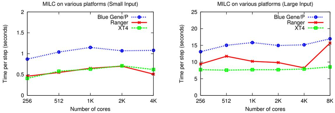
Figure 10: Performance (weak scaling) of MILC on the three machines
