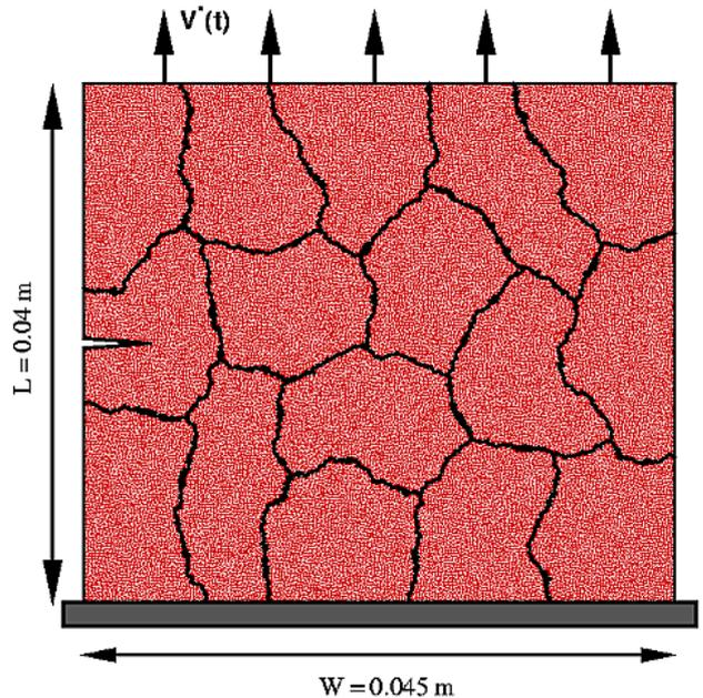
**Fig. 6** Initial mesh, boundary conditions and inter-processor boundaries for the parallel adaptive finite element simulations of a dynamic fracture event. The initial crack length  $a_0 = 0.005m$ .
