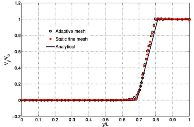
**Fig. 3** Vertical velocity distribution along  $x = 0$  at  $C_d t/L = 0.3135$  obtained analytically (solid curve) and numerically (symbols) for the 1D wave problem shown in Figure 2. The mesh adaptivity parameters are  $\epsilon = 0.75$  and  $\Delta t_{adaptive}/t_{ramp} = 0.25$
