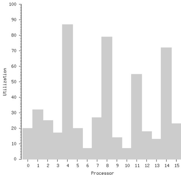
**Fig. 20** Processor utilization during mesh refinement in the adaptive phase of the dynamic failure problem solved on 16 processors.
