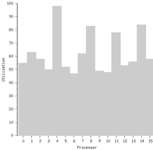
**Fig. 13** Processor utilization in the computation phase of the dynamic fracture problem on 16 processors while using block mapping
