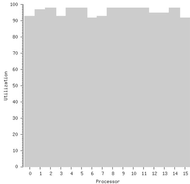
**Fig. 17** Processor utilization in the computation phase of the dynamic failure problem on 16 processors after load balancing.
