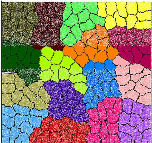
**Fig. 11** The adapted mesh used in the dynamic fracture problem is divided among 160 virtual processors. The dark lines indicate partition boundaries. The region of higher mesh density indicates the location of the stress wave.
