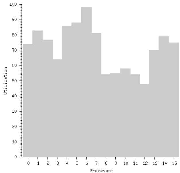
**Fig. 15** Processor utilization in the computation phase of the dynamic fracture problem on 16 processors with round-robin mapping.
