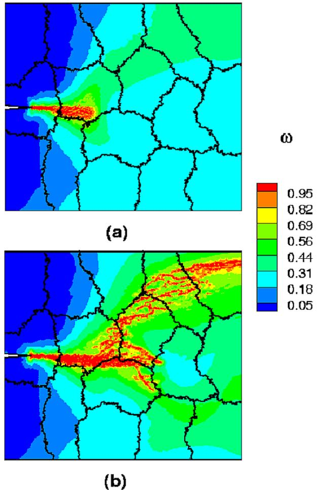
**Fig. 9** Damage parameter  $\omega$  distribution for the dynamic fracture problem shown in Figure 6 at (a)  $t = 2.613L/C_d$  and (b)  $t = 4.180L/C_d$ .
