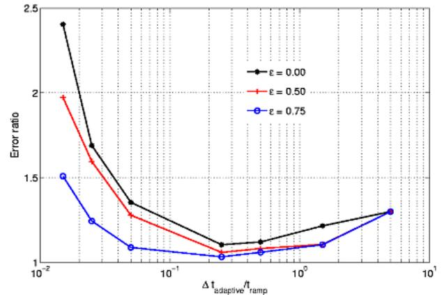
**Fig. 4** Comparison between the numerical error on the  $y$ -velocity field associated with the adaptive and static simulations for the 1D wave propagation problem shown in Figure 2: effect of the mesh adaptivity parameters  $\epsilon$  and  $\Delta t_{adaptive}/t_{ramp}$ . The error defined by (12) is computed at  $C_d t/L = 0.314$ .
