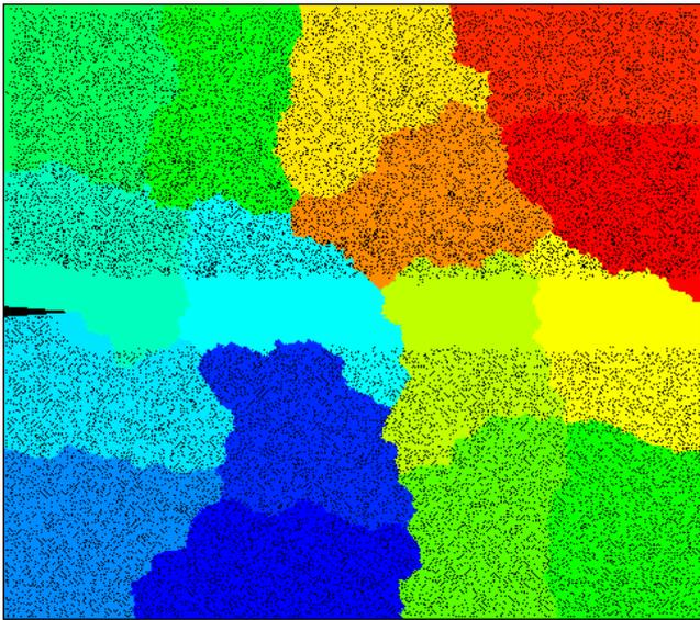
**Fig. 12** Finite element mesh after 10,000 timesteps of the dynamic fracture problem. There are 160 virtual processors mapped to 16 processors using block mapping. Different shades indicate different processors.
