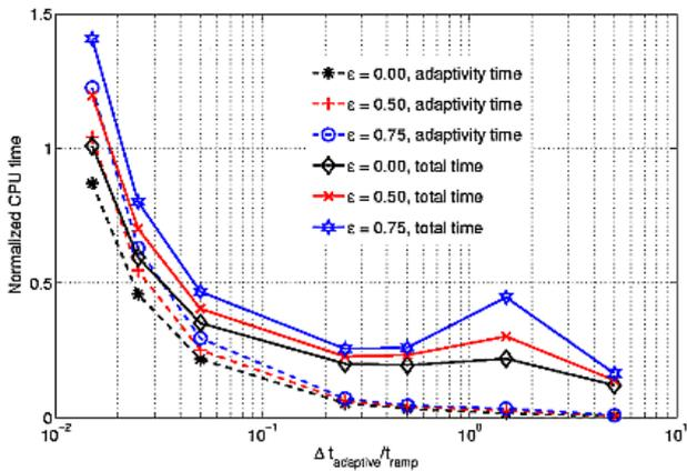
**Fig. 5** Effect of the mesh adaptivity parameters  $\epsilon$  and  $\Delta t_{adaptive}/t_{ramp}$  on the computational cost of the adaptive simulations for the total time (solid curves) and the CPU time dedicated to the mesh refinement and coarsening operations (dashed curves) for the 1D wave propagation problem shown in Figure 2. The CPU times are normalized by the total CPU time associated with the fine static mesh simulation.
