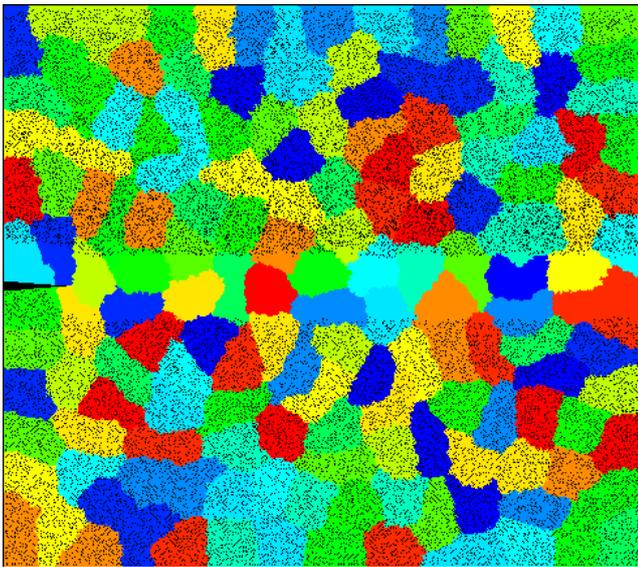
**Fig. 16** Adapted mesh after 10,000 timesteps with 160 virtual processors mapped onto 16 processors. The greedy strategy was used to perform load balancing after the mesh modification phase. Different shades indicate different processors.
