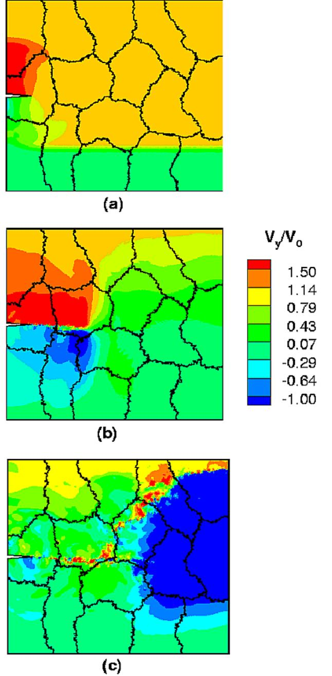
**Fig. 8** Normalized vertical velocity  $V_y/V_0$  distribution at times (a)  $t = 0.783L/C_d$ , (b)  $t = 2.613L/C_d$  and (c)  $t = 4.180L/C_d$ .
