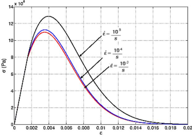
**Fig. 7** Stress-strain curve under uniaxial state of strain obtained for  $p_1 = 10$ ,  $p_2 = 0.8$ ,  $Y_{in} = 6000\text{J}/\text{m}^3$  and for various strain rates  $\dot{\epsilon}$ .
