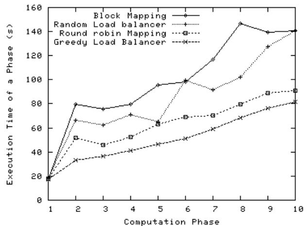
**Fig. 18** Execution time for each computation phase of the dynamic fracture problem for block mapping, round-robin mapping, random load balancer and greedy load balancer. Each computation phase lasts for 2000 timesteps and is followed by a mesh modification phase. The data is shown for a run with 160 virtual processors on 16 processors.
