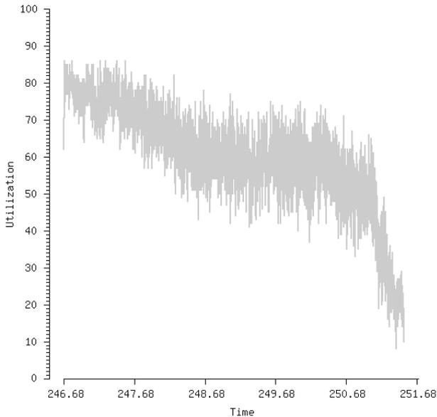
**Fig. 23** Processor utilization over time during refinement in the adaptive phase of the dynamic failure problem on 16 processors after pre-balancing.
