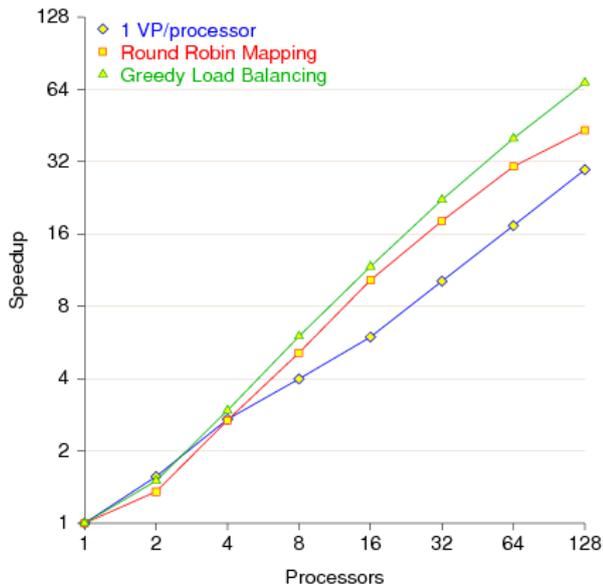
**Fig. 19** Scaling results vs. best single processor execution time.
