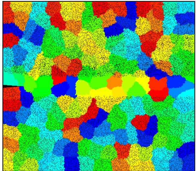
**Fig. 14** Mesh after 10,000 timesteps with 160 virtual processors mapped onto 16 processors using round-robin mapping.
