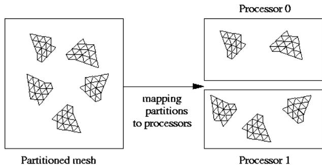
**Fig. 1** The CHARM++ run-time system maps virtual processors to physical processors. In ParFUM, each virtual processor is associated with one partition of the mesh.
