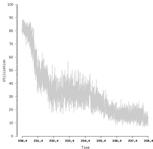
**Fig. 21** Time evolution of processor utilization during mesh refinement in the adaptive phase of the dynamic failure problem solved on 16 processors.
