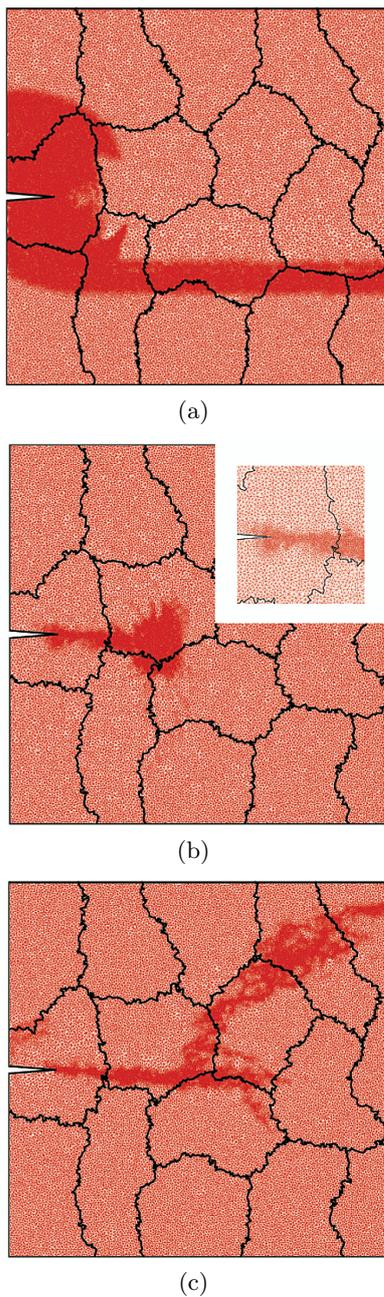
**Fig. 10** Adaptive mesh for the dynamic failure problem shown in Figures 8 and 9 at (a)  $t = 0.783L/C_d$ , (b)  $t = 2.613L/C_d$  and (c)  $t = 4.180L/C_d$ . The inset figure shows details of the refined mesh in (b) in the vicinity of the notch tip.
