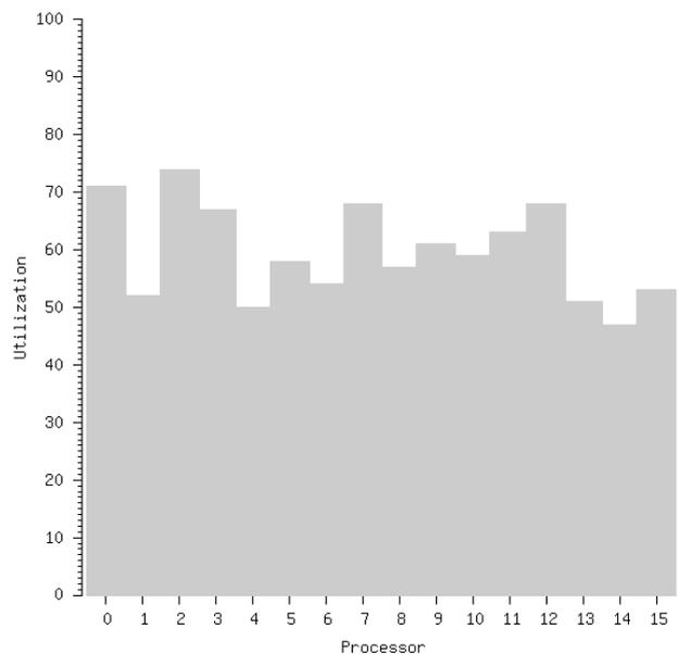
**Fig. 22** Processor utilization during refinement in the adaptive phase on 16 processors after pre-balancing.
